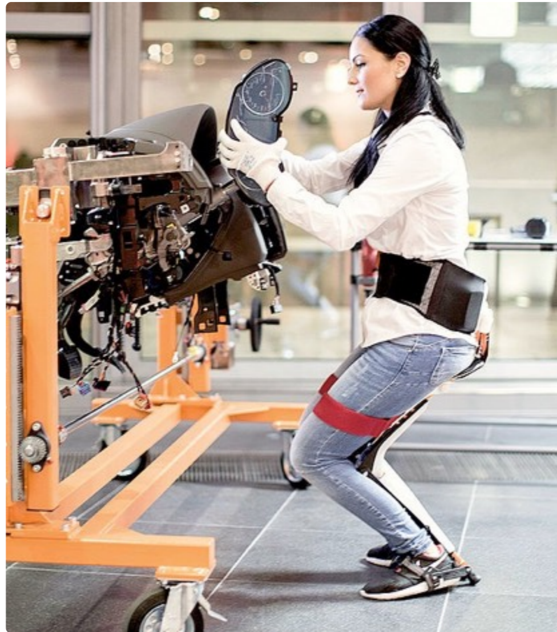
Chairless chair exoskeleton system to relieve workers fatigue. Image credit: Noonee
