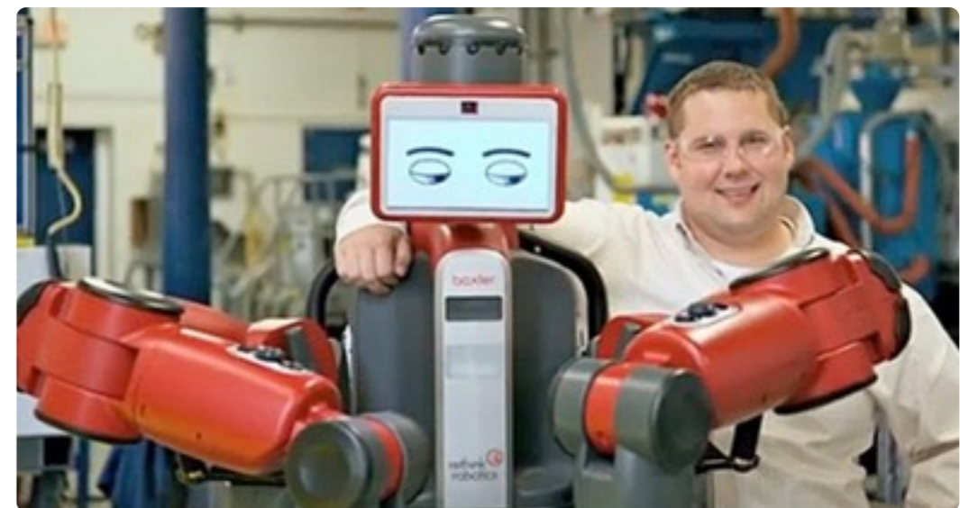
Baxter has been designed to operate in human teams as a co-worker. It can learn by looking at its co-workers and can even teach them new improved ways to cooperate. Image credit: Rethinking Robotics
