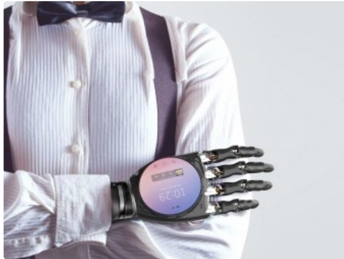
A smart prosthetic hand that goes beyond the functional replacement of the lost hand. Through a computer and a display it can become a communications gateway. Image credit: Jung Jo In
