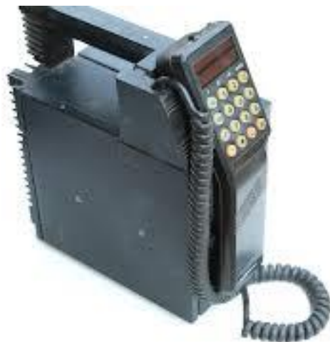
Figure 6. An early “mobile phone”. This device was more like a suitcase than the small, slick phone we are accustomed to fitting in our pocket/purse. The big box contained both the electronics and the battery, both pretty bulky! Image credit: eBuyer
