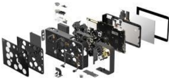
Figure 10. The L16 has 16 lenses, each time you take a photo you are using several of them, and software takes care of fusing the individual lens output into a single photo. Image credit: Macfilos
