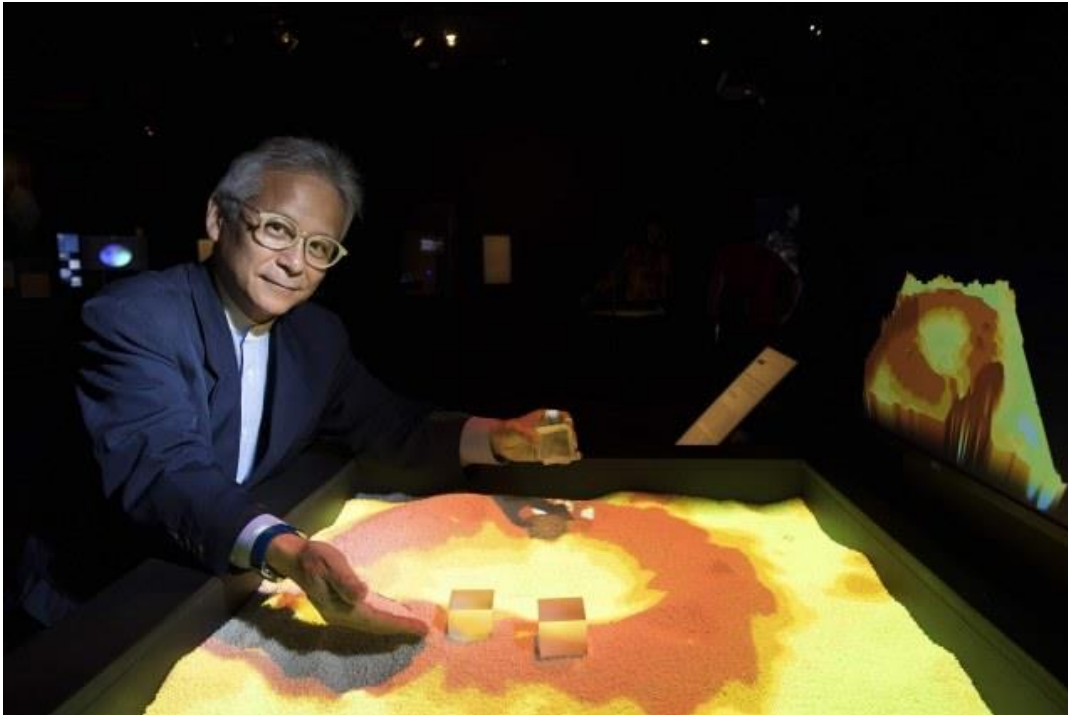
Figure 12 Hiroshi Ishii has been leading research on Tangible Interfaces. One of the applications is the design of internet networks using digital modelling and SandScape, a broad surface covered with sand. By moving the sand and placing objects on the sand representing network equipment, one could experiment the effect of different architectures. It was a mixture of digital and physical reality used to grasp the effect on a “different” physical reality. Image credit: Media Lab
