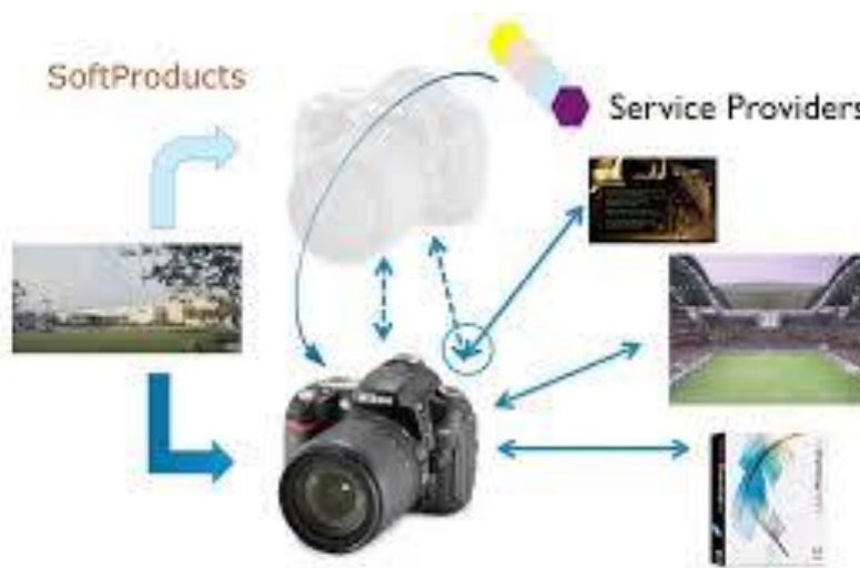
Figure 9 A graphic from several years ago used to explain the trend towards product softwarization. In this case a digital camera operates using embedded software that can be updated and extended both by the camera producer as well as by third parties. This software is both the engine of the digital camera and a platform delivering features and services. The end user seldom perceives what feature is hardware based and what feature is software based.
