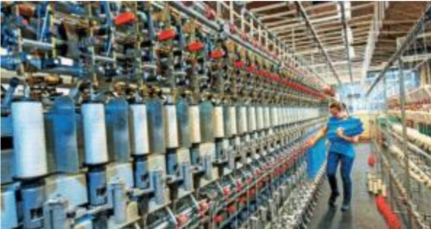
Figure 19 Textile manufacturing involves very sophisticated and extensive plants having multiple hundred thousand components (320,000 bearings, 1,250 motors, 3,500 transmission belts, 50,000 spindles to produce 43,000 kg of fabric a day). Downtime is extremely costly and can kill margin. Image credit: Indian textile journal
