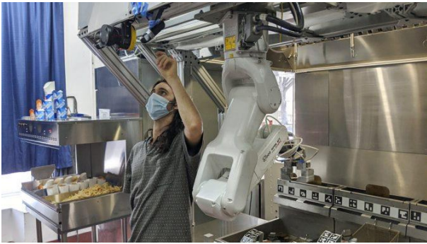
Fig. 87 Flippy, a kitchen robot for fast food restaurant can prepare burghers and salads. Demand is expected to grow as restaurants face Covid-19 restrictions. Image credit: Miso Robotics, California
