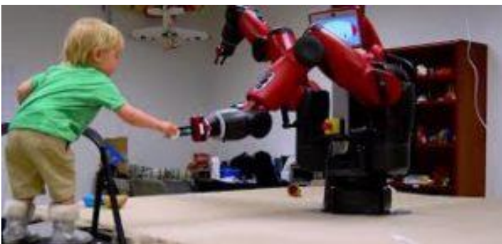
Fig. 23 Baxter, the collaborative robot, is shaking hands with a little kid. It was designed to work along with humans and to learn from them. Image credit: Rethinking Robotics
