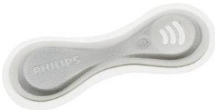
Fig. 74 A self-adhesive biosensor that automatically and continuously measures vital signs, body posture and step count, and detects falls. Image credit: Philips
