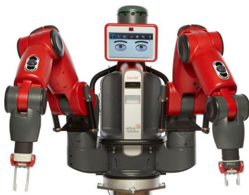
Fig. 110 The Baxter co-bot has been designed with some anthropomorphic traits—a screen is used as a head to convey a sense of attention, emotion, etc. Image credit: Rethink Robotics
