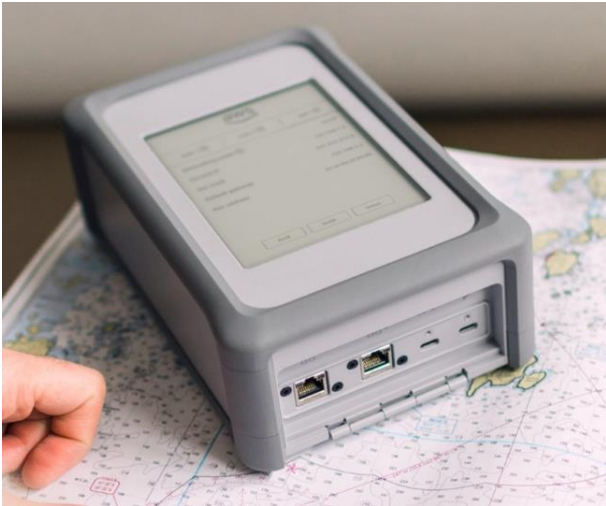
Figure 30. Amazon Snowcone is a rugged box designed to provide edge computing in the field, extending the AWS services at the edge by creating a local cloud with processing capability. Image credit: Amazon
