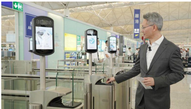
Figure 3. Facial recognition at the Hong Kong Airport. The image picked up by the videocamera at the gate is matched with the one stored in the passport chip to check the person's identity. Image credit: Hong Kong Airport Authority
