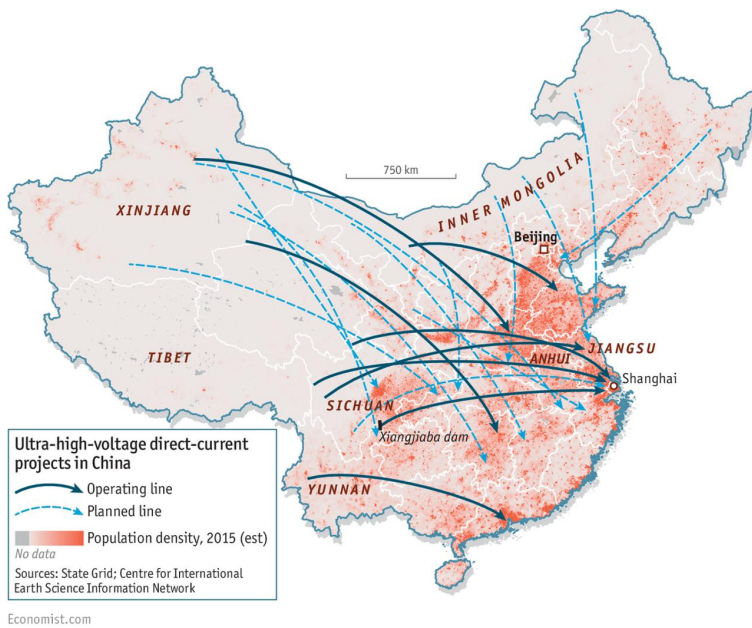
Figure 53. Active and projected UHVDC infrastructure in China. Notice the very long span of the power lines connecting deserted areas to cities where electrical power is needed. Image credit: the Economist
