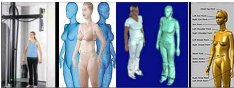
Figure 13. A 3D full body scanner can take precise measure of your body and create a digital replica that can be used in manufacturing custom apparels. Image credit: Fibre2Fashion
