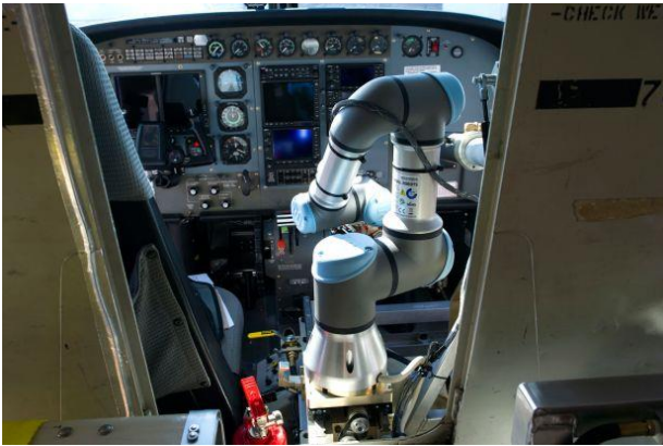
Figure 38. A robot is sitting on the pilot seat. There are already a number of airplanes that are able to fly and land in an autonomous way (departure remains tricky) but for airplanes without this capability a robot impersonating the pilot may do the job. Image credit: DARPA with Aurora Flight Sciences
