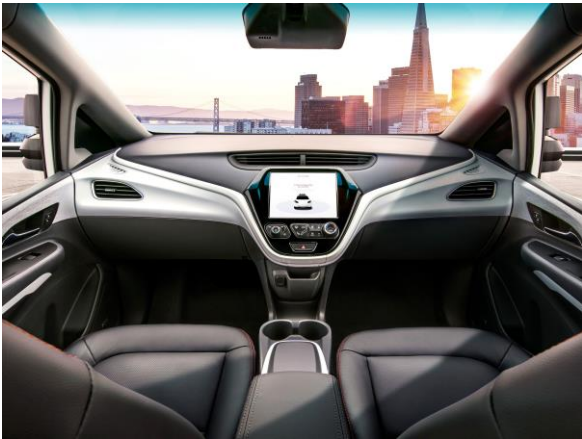
Figure 39. Missing something? This car has no steering wheel. That is the idea of car by General Motors. Image credit: GM
