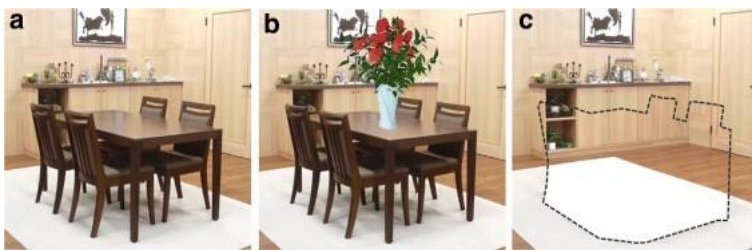
Figure 5. Augmented reality, adding a vase with flowers on a table, is “easy”. Diminished reality is difficult and partly magic, like removing the table and “creating” what the table presence was hiding. Image credit: Fayteq
