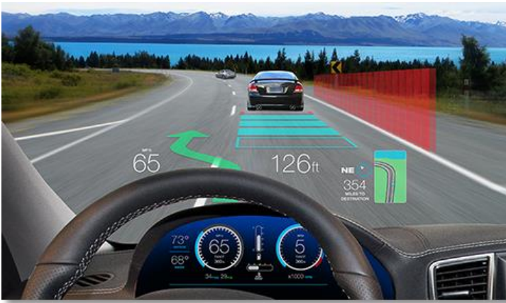
Figure 45. Head Up Display showing the distance from the vehicle ahead, the path leading to the overtaking and information on the road. More advanced HUD can display the full path, showing when the overtake will be completed and the car can return back to the original lane. Image credit: WardsAuto
