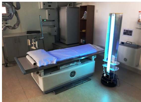
Figure 62. Violet is a robot designed to help in sanitation of hospital rooms and can be used in closed spaces like stores and in offices. Using UV light, it can kill the coronavirus and has a smart detection system to switch off the UV light if a human shows up. Image credit: Akara Robotics
