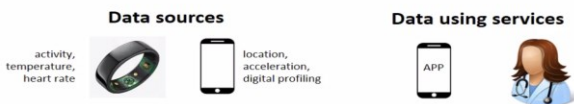
Figure 20. There are multiple personal data sources that can feed data to a PDT. Likewise, there can be several (interested) users for this data. Rather than having the data directly accessed by the users, the PDT can intermediate, thus maintaining control of sharing personal data. Hence the PDT becomes a crucial element in the data governance. Image credit: Juuso Autiosalo
